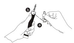
2.) Slide the exhausted battery out of the flashlight.
